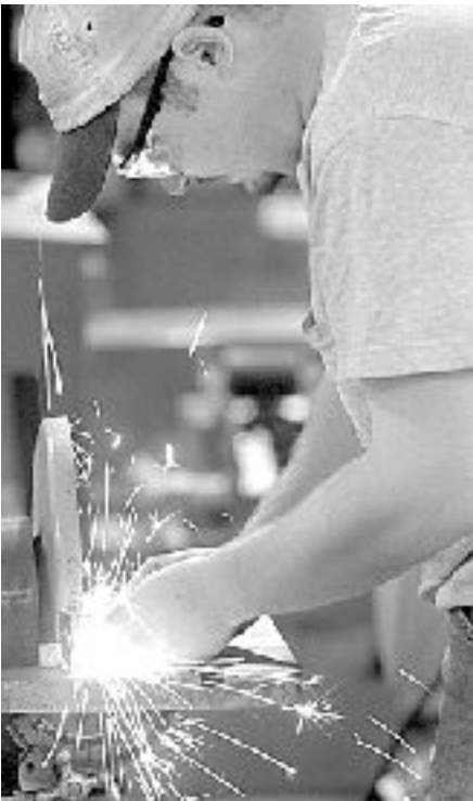
Production assistant James Belden, Concordia, uses a grinder to remove burrs from rivets Wednesday at G.L. Huyett Co.
