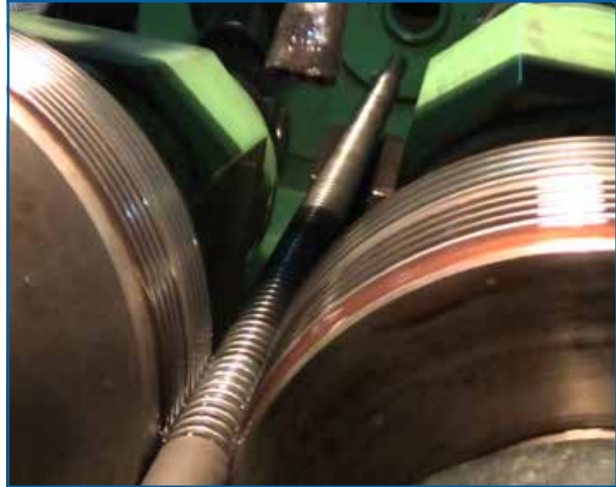
A thread rolling machine can cut right or left threads without retooling. Threading is used on parts that attach with either external or internal threads.
