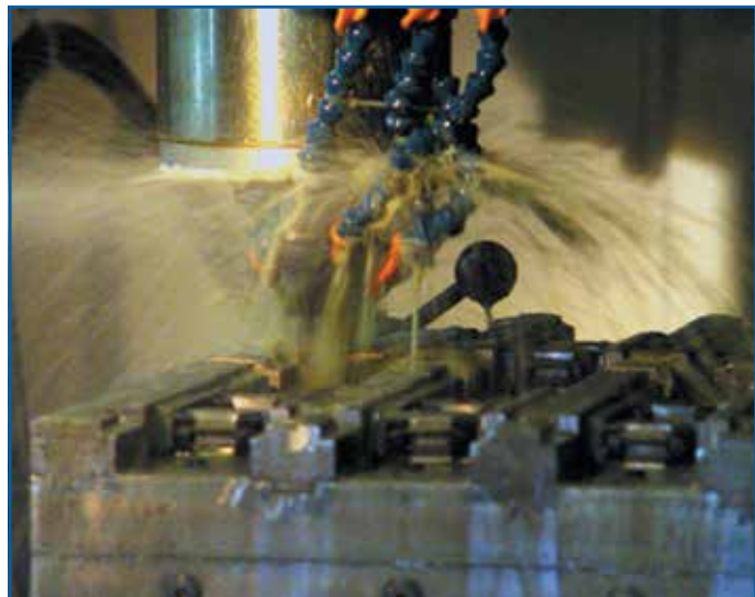
Milling uses a rotating cutter to create shapes such as gib keys and step keys from blocks of metal. Radiused ends and countersunk holes are also possible.
