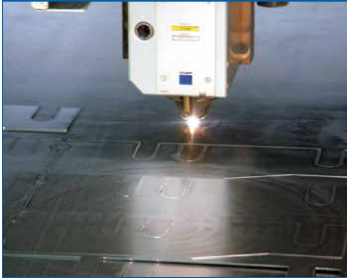
Laser drilling and cutting is a new technology replacing cutting and stamping when extremely accurate shapes are required. It is highly efficient on smaller quantity items such as prototypes as no tooling is required.
