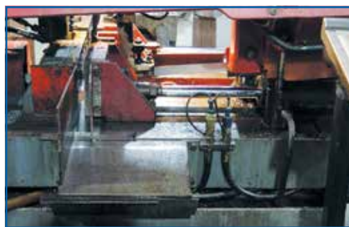
Cold-sawing is slower than band sawing, but is highly accurate and does not scar the metal. It is used to make products such as woodruff keys and spacers with keyways.
