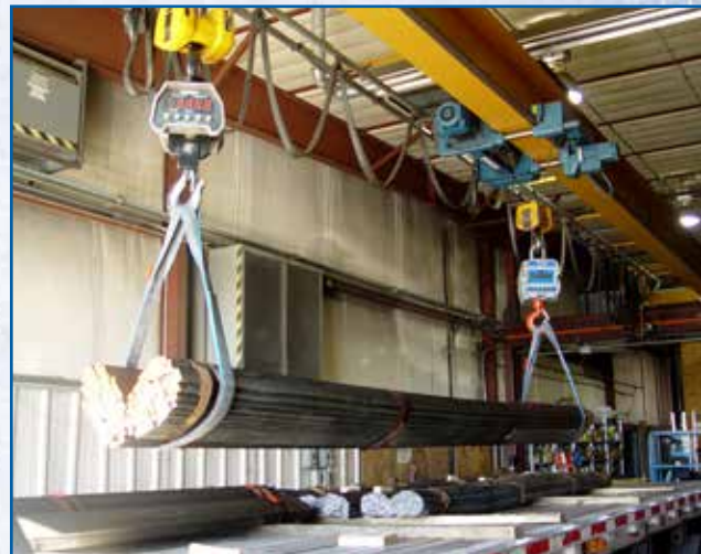
Full bundles of steel are lifted in two places to minimize bending, twisting, and contortion.
