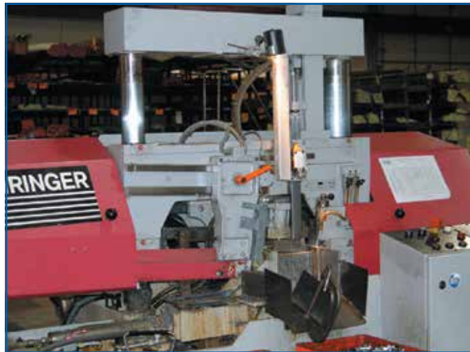
Automated industrial band saws are used to manufacture machine keys, keystock, and spacers to tight tolerances for a wide range of applications and industries.
