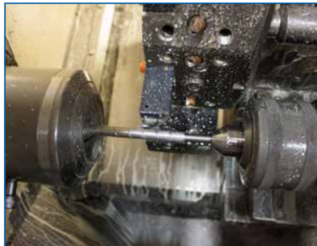
The workpiece is mounted into the chuck. As it rapidly spins, a cutting tool can shape the piece into a round form, cut grooves, or produce radiused corners.
