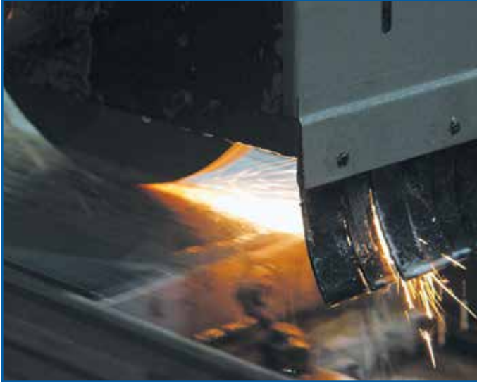
Grinding is employed when extremely tight tolerances are required on flat surfaces such as shims and thrust washers.
