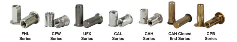
Blind Rivet Nuts provide load-bearing threads in thin sheet materials that are too thin for a tapped thread. They are called "blind" because they can be installed from one side of the work piece. Once the rivet nut is installed, additional components can be attached using threaded fasteners.
