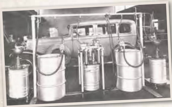
AN EARLY 1900'S LINCOLN® LUBRICATION SYSTEM
