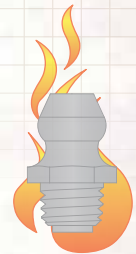
FITTING IS RE-HEATED TO SCALE BACK HARDNESS TO DESIRED SPECIFICATION.
